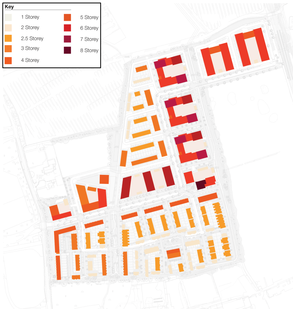
Figure 8: Extract from the Design Statement, prepared by O'Mahony Pike Architects illustrating height of the proposed buildings for the overall Masterplan (i.e. including Phase 1 and 2).
